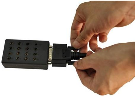
Connect the jumper box to the main test leads and tighten the fastening bolts as shown on the left. In the jumper box you can see 15 jumper connection holes, respectively marked with numbers, the numbers of these connection holes corresponding to the car OBD interface pins, as shown in Figure 4.2.3.2.
